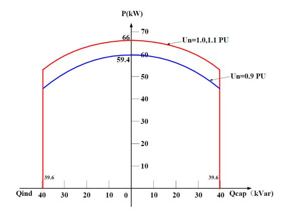
**Note:** When SUN2000-60KTL-M0 operates at grid voltage 1.0/1.1 p.u., the output power can reach 66kW (when PF=1) or 66kVA.
