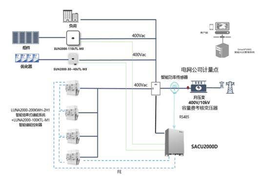
Huawei Industrial and Commercial Energy Storage Products which the LUNA2000-200kWH-2H0 and LUNA2000-200kWH-2H1 (ESS for short) are applicable to industrial and commercial scenarios. The LUNA2000-200kWH-2H1 works with the SmartPCS, DCDC, and SACU. The SmartPCS is connected to the cluster controller DCDC, and charges batteries when the power grid is sufficient. When the power grid needs to be output, the SmartPCS outputs the stored battery energy to loads for use.
