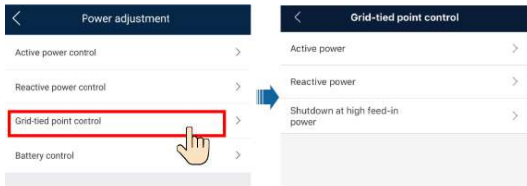
Figure 7-7 Grid-tied point control
