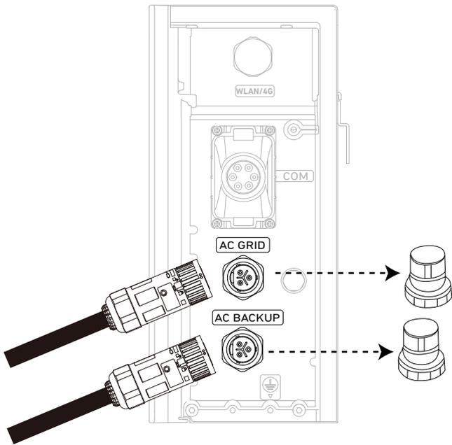
10. Connect the AC grid cable to the main panel, and the AC backup cable to the subpanel.
