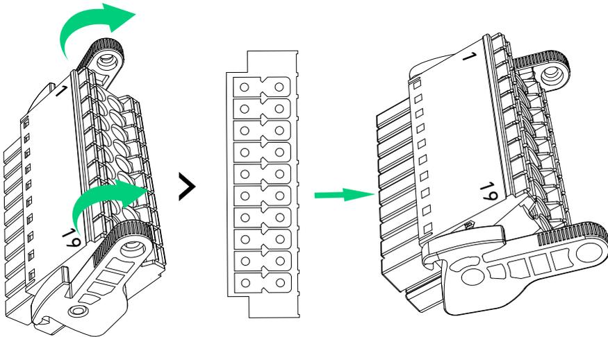
6. Insert the wiring compartment cover by pressing the clips on both sides and tighten the locking cap.
