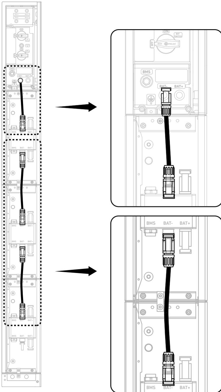
5. Connect the positive DC power cables between the modules.
