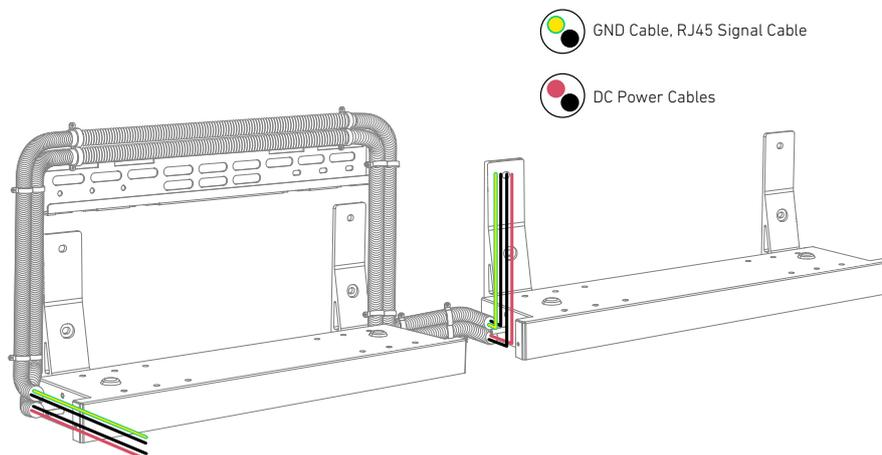
② Assemble the GND cable and RJ45 signal cable.
