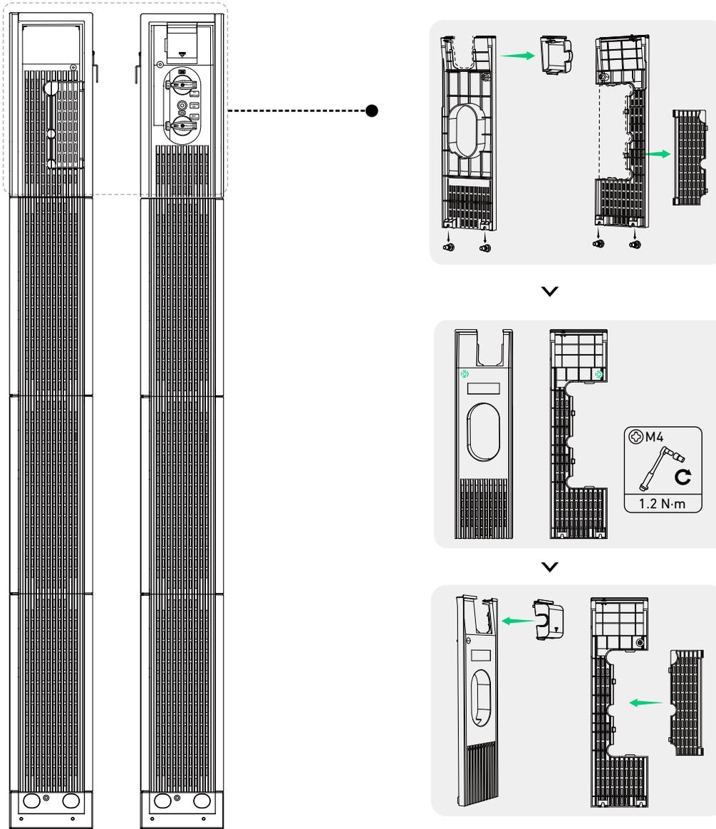
3. Attach the baffles to the modules.
