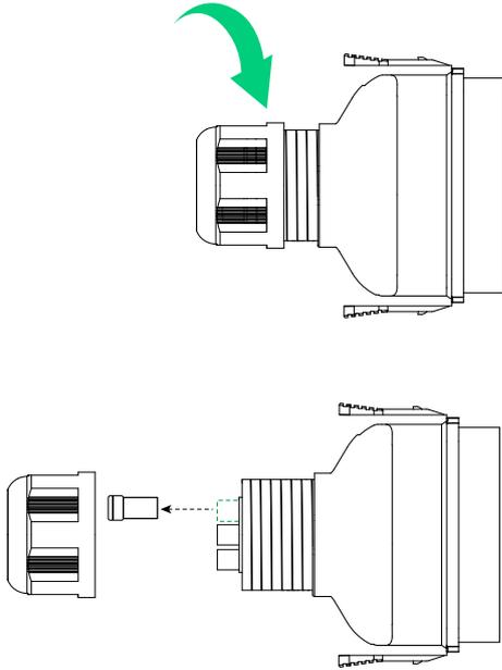
3. Route the 2-wire RS485 signal cable ( $5.5 \pm 0.5$  mm in outer diameter, included) through the locking cap and wiring compartment cover.
