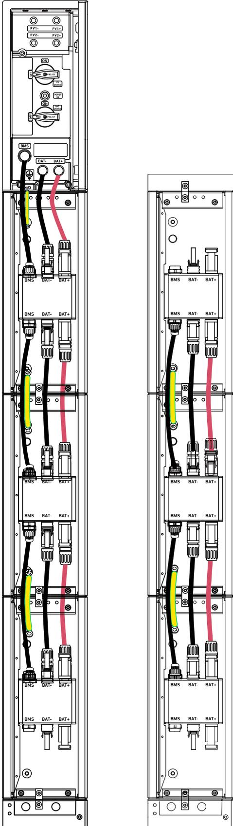
2. Connect cables between the bottom modules.
