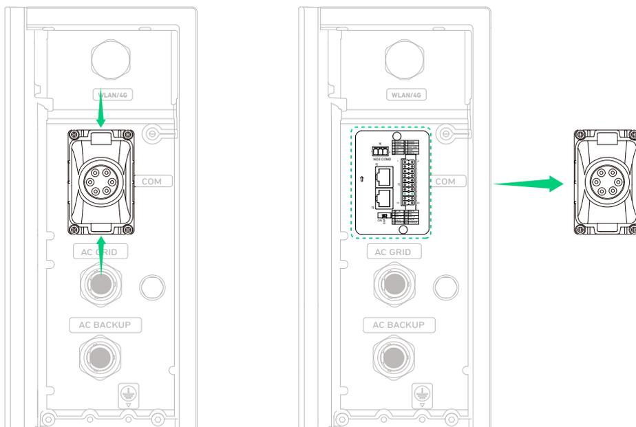
2. Rotate to remove the locking cap from the wiring compartment cover and take out a waterproof plug.
