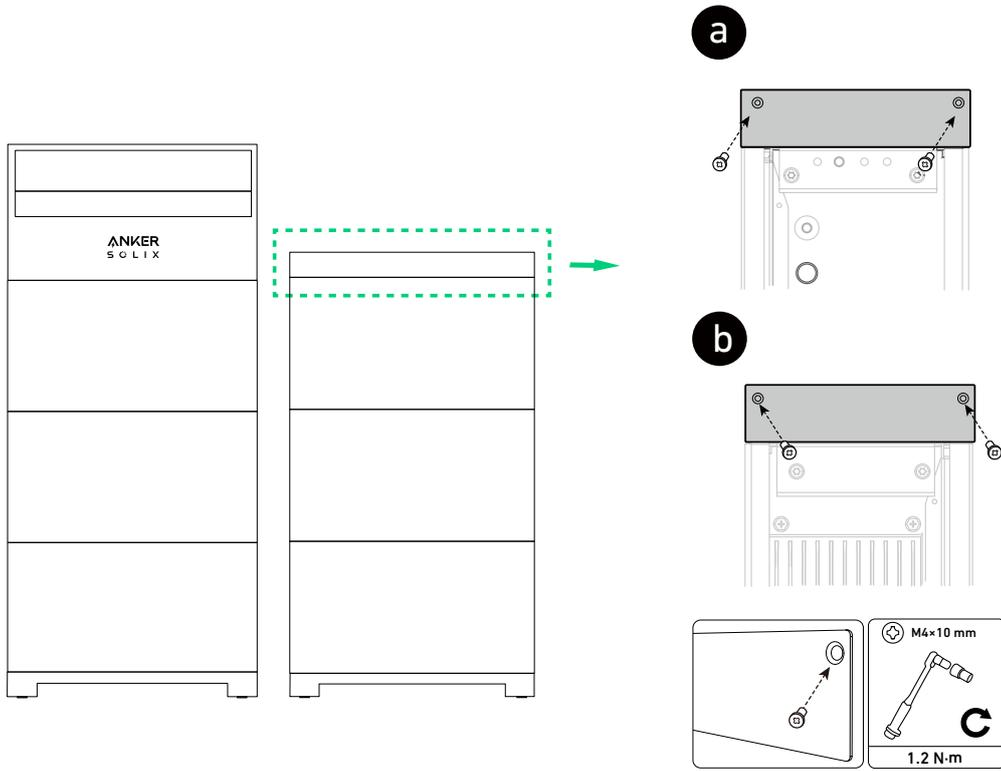
② Attach the base baffles to the battery module base in the first column. Make sure the baffle side with the countersunk holes face outward and tighten the screws.
