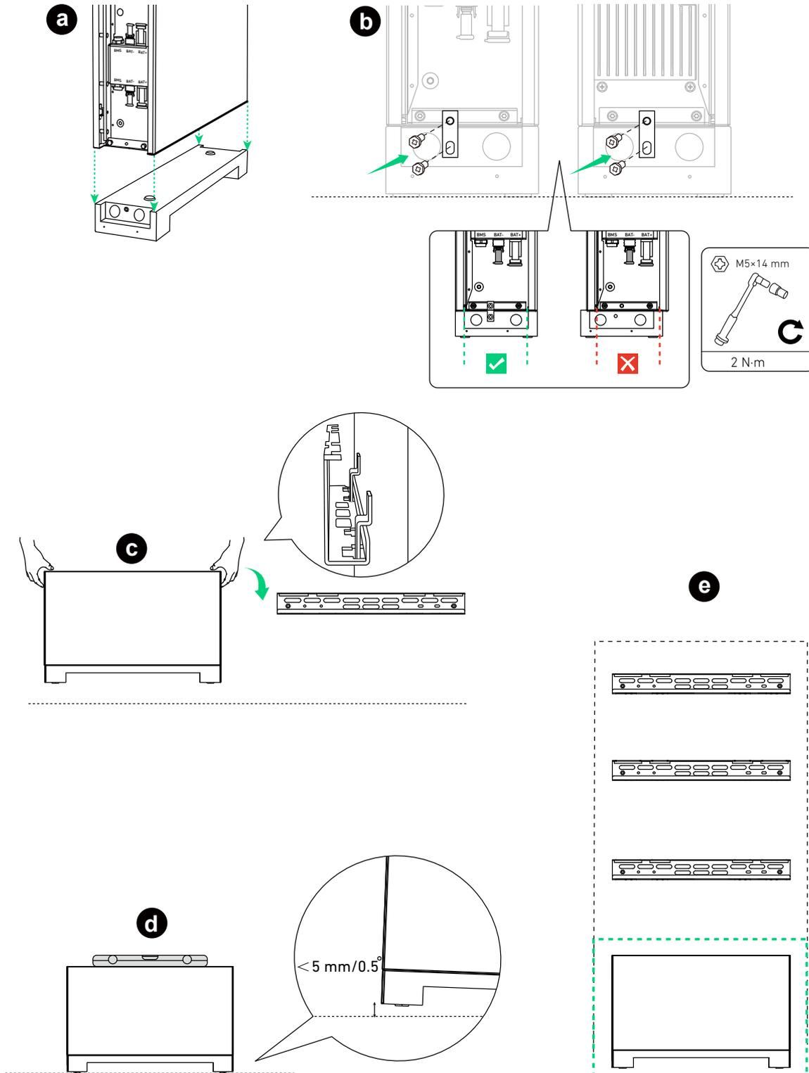
2. Mount the remaining power module and battery modules from bottom to top.
