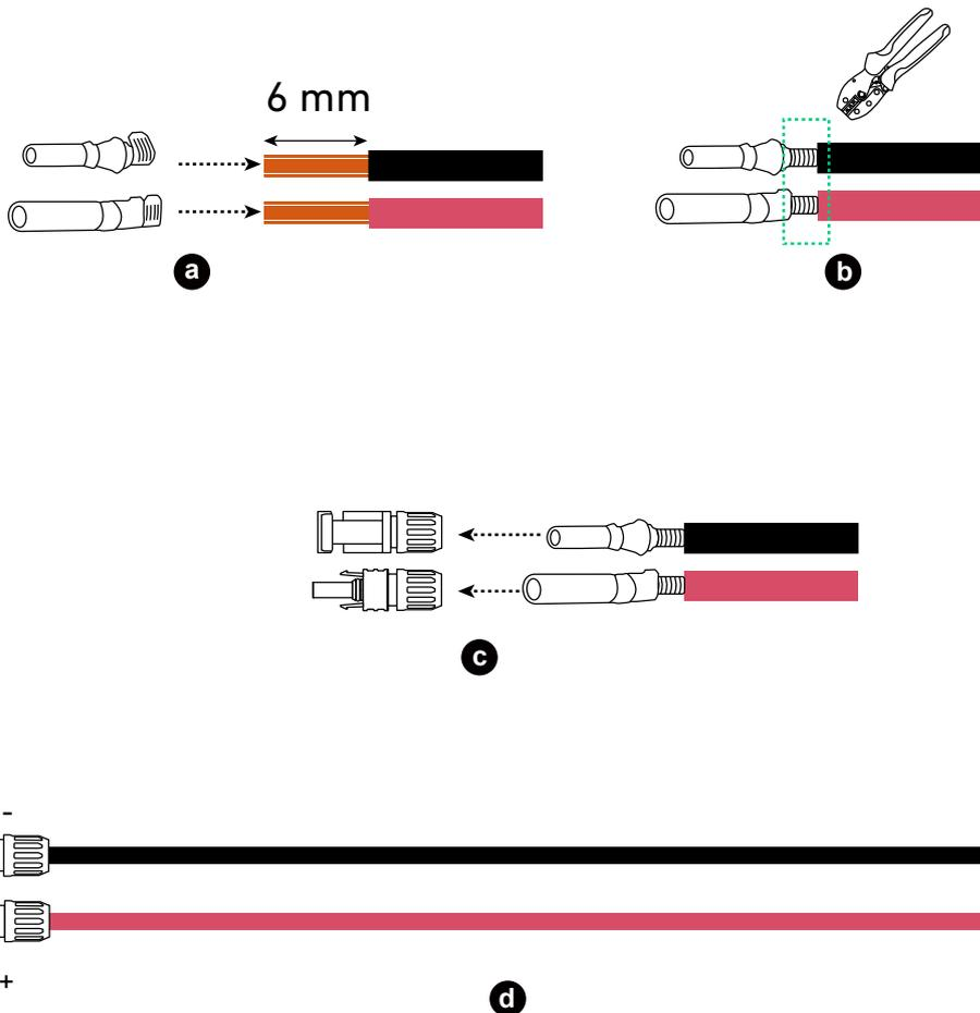
3. Connect the positive PV connector to a positive PV power port (PV1+ or PV2+) and the negative PV connector to a negative PV power port (PV1- for PV1+, or PV2- for PV2+).
