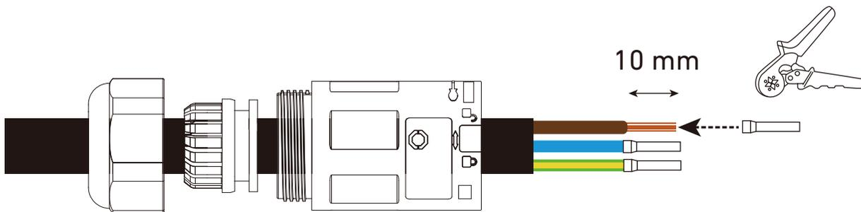
4. Connect the live, neutral, and PE conductors to the sockets labelled L, N, and PE respectively.
